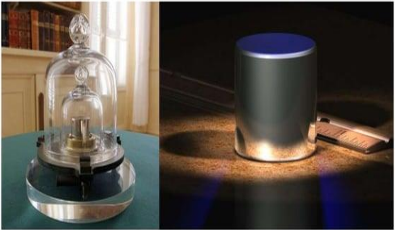
Prototype cylinder of platinum-iridium alloy
